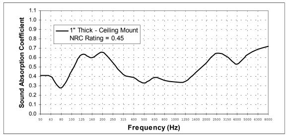
Note: Tested per ASTM C423
