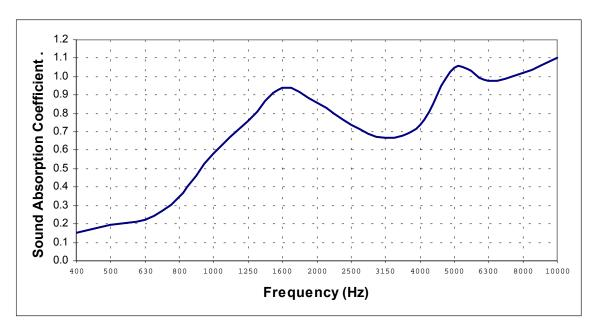
Note: Test Sample Thickness = 30 mm (1.2") Alpha Cabin Measurements
